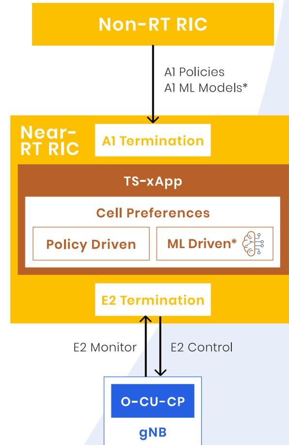
Figure 2. The deployment of TS-xApp within the O-RAN architecture.
