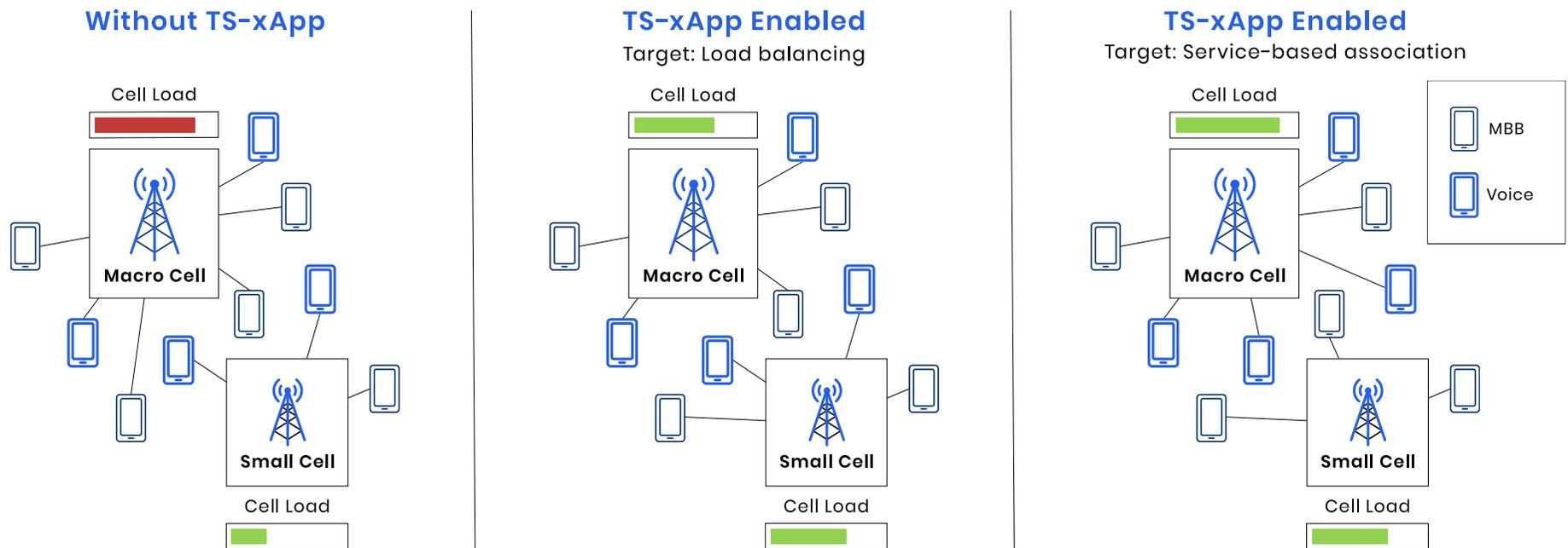
Figure 1. Example of TS-xApp operation
