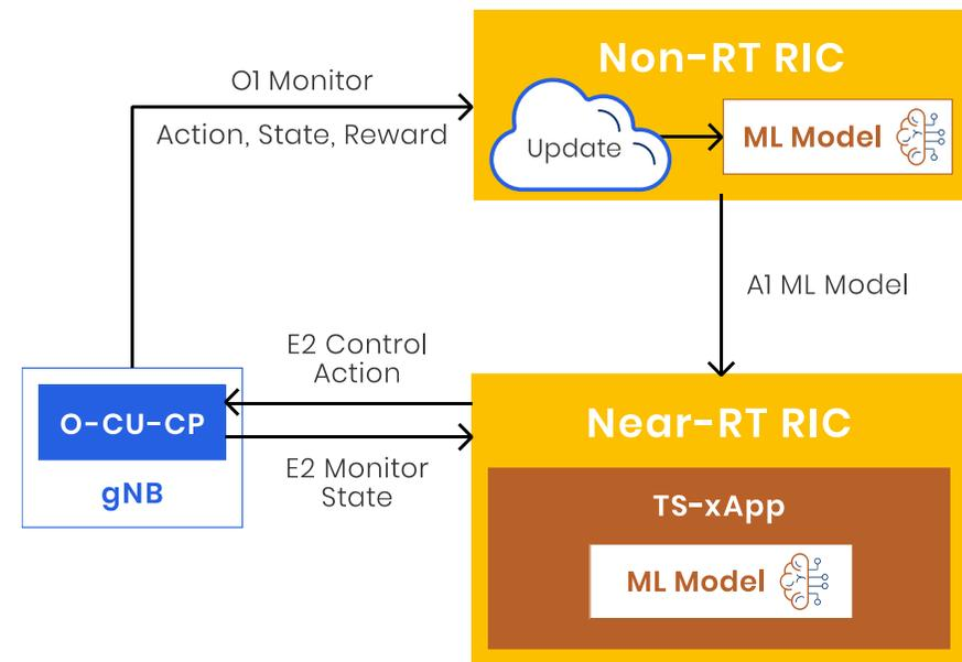
Figure 4. The Machine Learning-Driven resource allocation in TS-xApp
